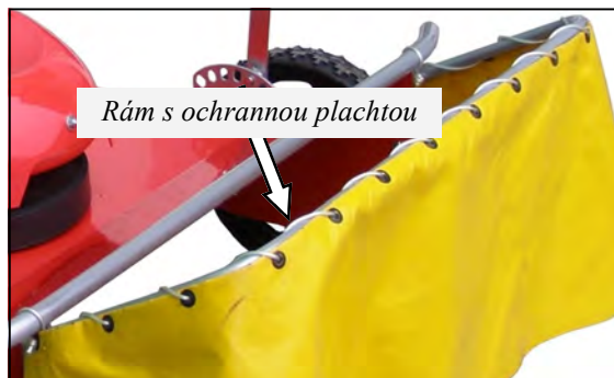
Obr. 43a,b,c Ochranná plachta mulčovače
